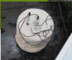
Static chambers for measuring the soil respiration and the net ecosystem exchange (NEE). © F. Laggoun
