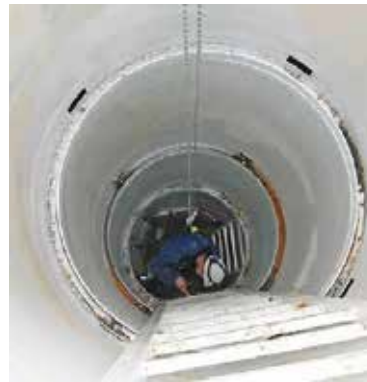
Example of an observation well set up in the vadose zone in New Zealand. © Close et al., 2012.
